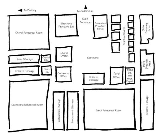
An effective floor plan provides adequate space for vocalists and instrumentalists, who need room to perform. The space also accommodates equipment, storage, and heavy student traffic, as well as the necessary cubic volume for proper acoustics.
