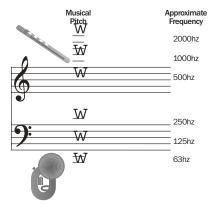
The sound frequencies produced by different instruments react differently when they come into contact with different surfaces. Flutes and violins, for example, produce high frequency sounds which are easily absorbed by a wide variety of common materials. Tubas and drums, on the other hand, produce low frequency sounds that are more difficult to absorb; they also produce easily absorbed overtones in higher frequency ranges that are critical to good intonation.
